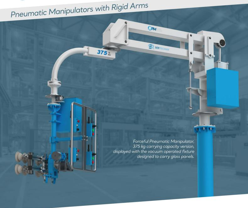
Forceful Pneumatic Manipulators are designed to move operator-centered loads within the work area with minimum effort. It balances the weight of the load, allowing the operator to carry the load quickly and safely.
